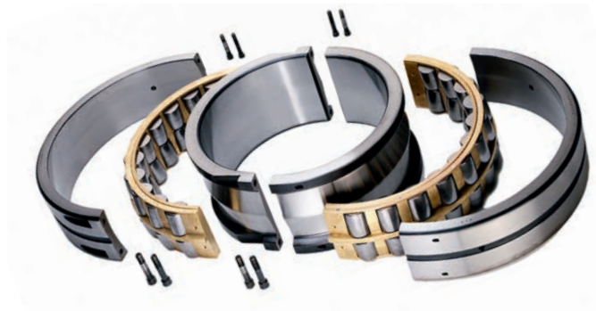
Exploded view of an FAG split spherical roller bearing with split solid cage made from glass fiber reinforced polyamide or brass; integrated locking rings
