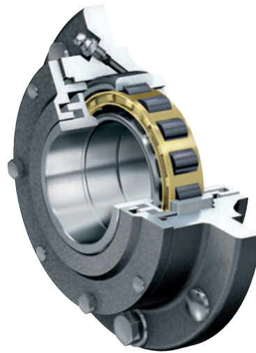
61 FKB housing unit with relubrication facility for traction motors
