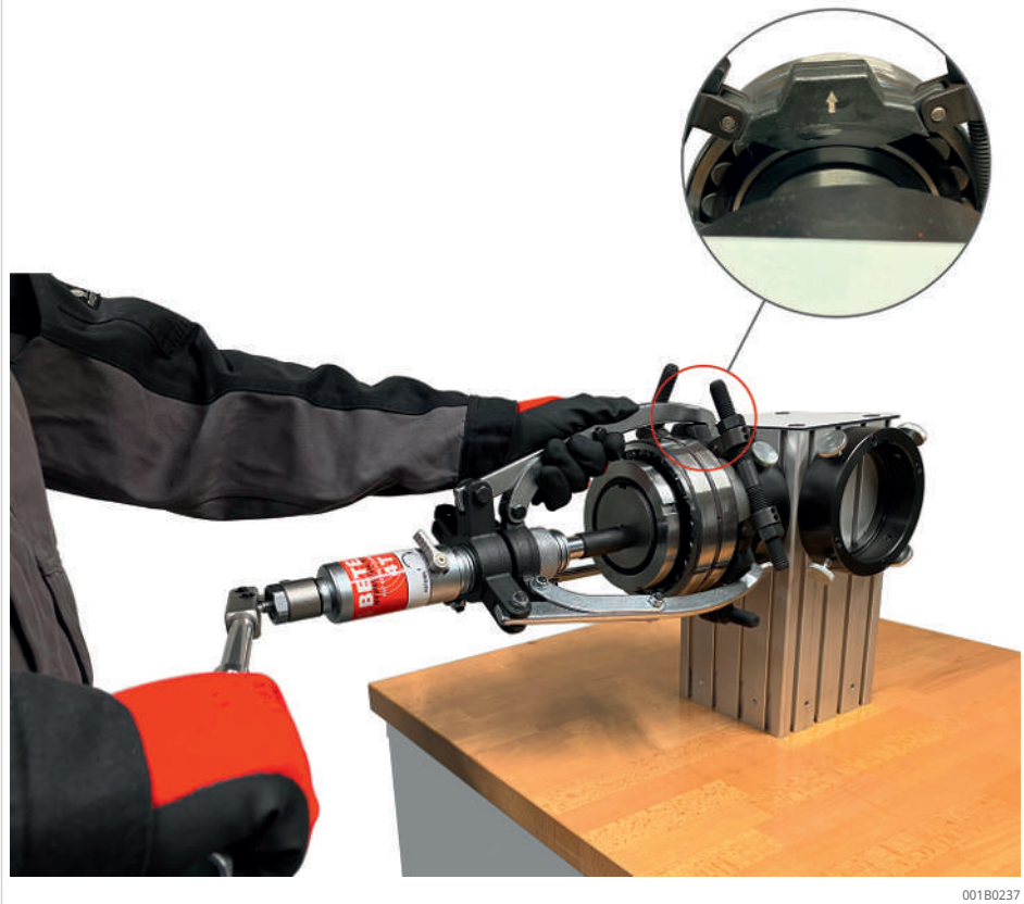
28 Dismounting with the TRI-SECTION-PLATE
