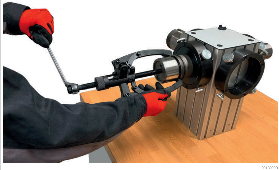
10 Use of the mechanical puller MSP-2/3
