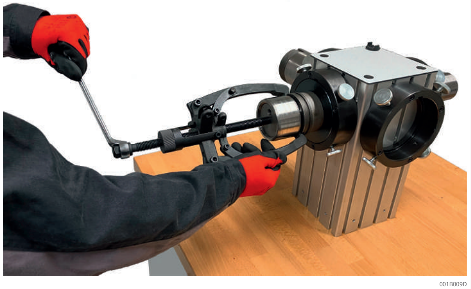
2 Use of the mechanical puller MSP-2/3
