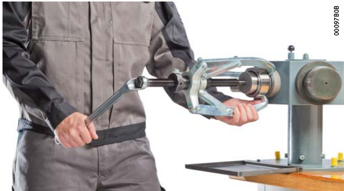
Figure 2 Use of the three-arm extractor PULLER-3ARM
