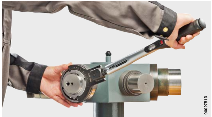
Figure 3 Use of the double hook wrench LOCKNUT-DOUBLEHOOK
