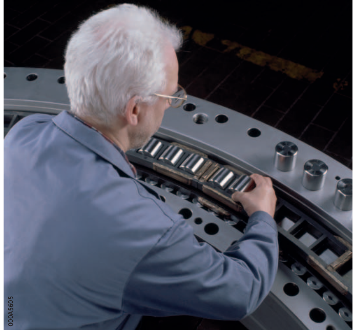
Figure 1 Fitting of rolling elements during reconditioning of a rolling bearing for a tunnel boring machine
