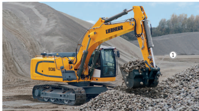
27 Application example with high wear load: Spherical plain bearing in excavator
