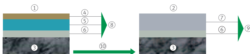
51 Coating systems for bipolar plates with and without a precious metal content
