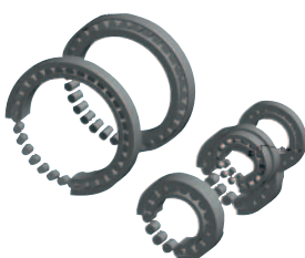
Figure 5: Generation of the calculation model including free bodies and shafts
