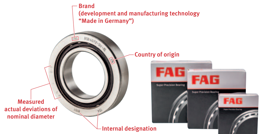
Figure 6: Marking of bearings
