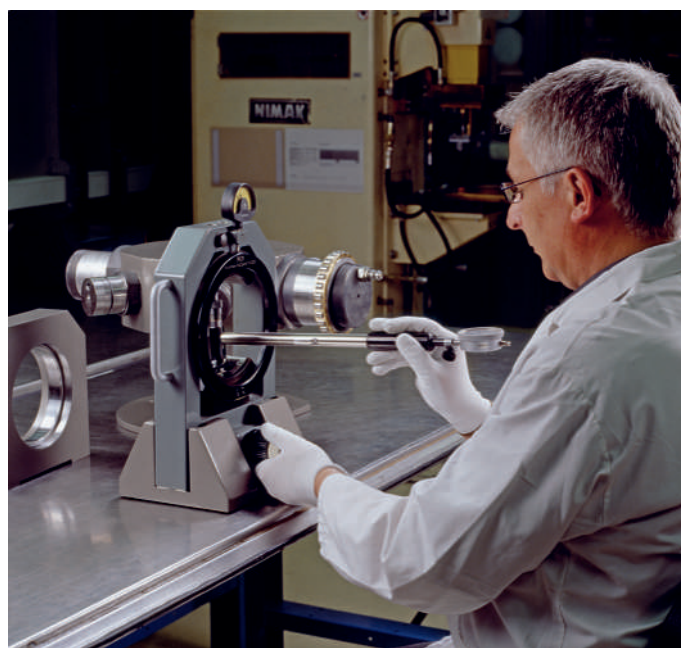
33 Transferring the raceway diameter to the enveloping circle gauge
