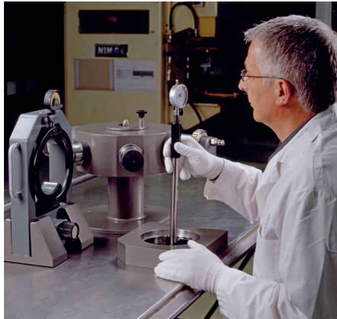
32 Measuring the raceway diameter of the outer ring
