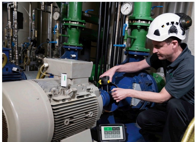
Industrial tools – Alignment Industry: LASER-EQUILIGN2 always ensures professional alignment of your machines thanks to single laser technology
