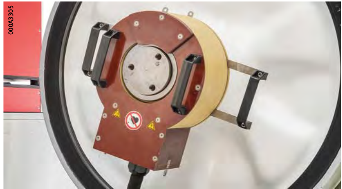
Figure 6 Dismounting of bearing inner rings of wheelset bearings (rail vehicles) using rigid inductor
