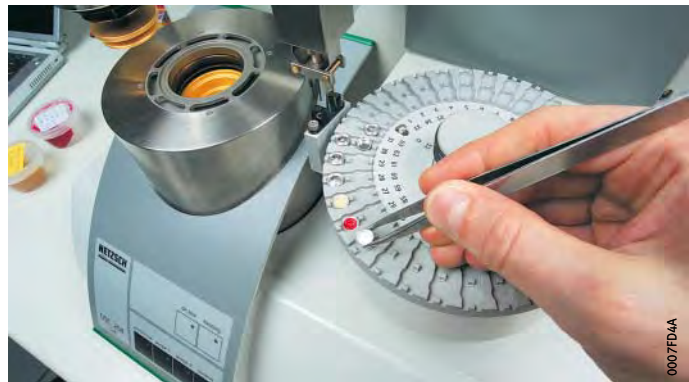
Figure 5 Analysis of the thermal behaviour of greases
