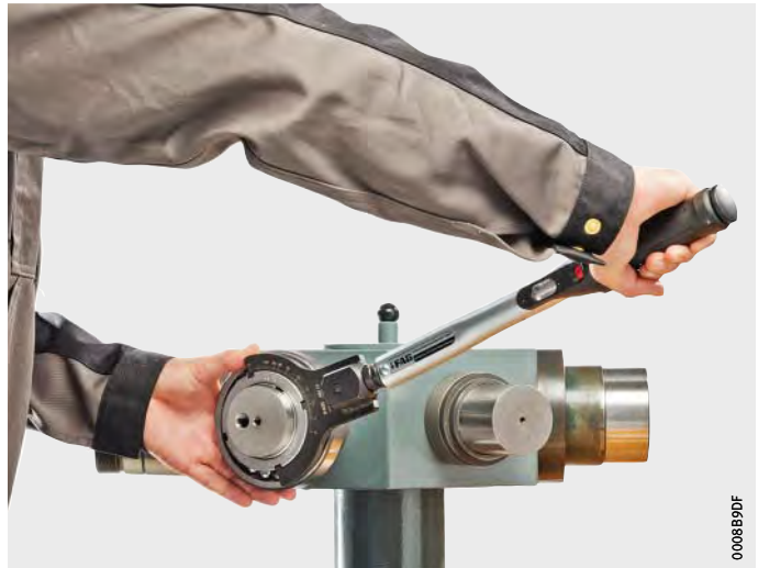
Figure 11 Mounting by means of double hook wrench
