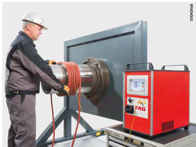
Figure 5 Dismounting of bearing inner rings using flexible inductor
