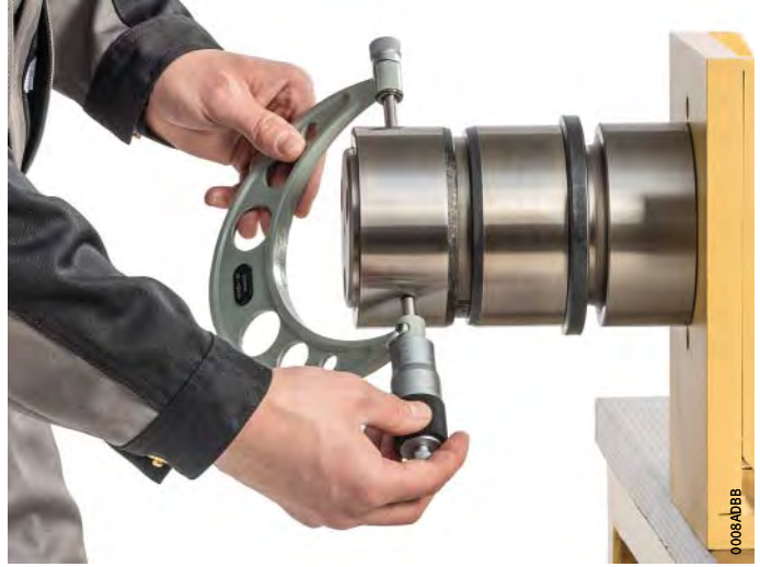
Figure 3 Measurement of expansion using external micrometer
