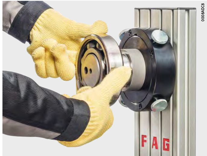
Figure 14 Sliding into place of heated bearing parts
