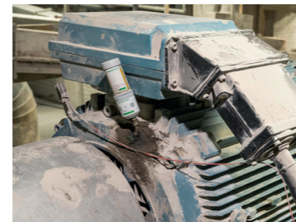
Cement: OPTIME C1 lubricates with pinpoint accuracy and, thanks to smart technology, always indicates the status on a (mobile) end device regardless of location
