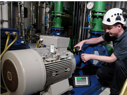
Industry: LASER-EQUILIGN2 always ensures professional alignment of your machines thanks to single laser technology
