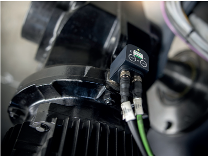
Logistics center: SmartCheck monitors rack feeder motors
