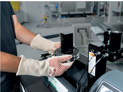
Industry: through gentle inductive heating, HEATERs prevent damages such as uneven running, fractures or abrasion marks
