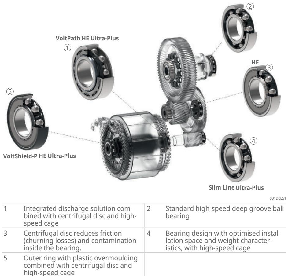
In addition to conventional high-speed deep groove ball bearings, the e-bearing Family includes additional features. These features can be combined as required to create an optimal bearing solution for the specific application.
