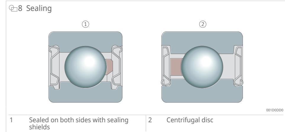
For applications in which the bearings operate in an oil bath, bearings in the HE design variant with centrifugal discs are available by agreement. The centrifugal disc reduces oil churning losses. Ideally, the centrifugal disc should be positioned on the side facing the oil. This arrangement reduces bearing friction and helps keep oil temperatures low. In addition, the centrifugal disc protects the bearing against contamination.
