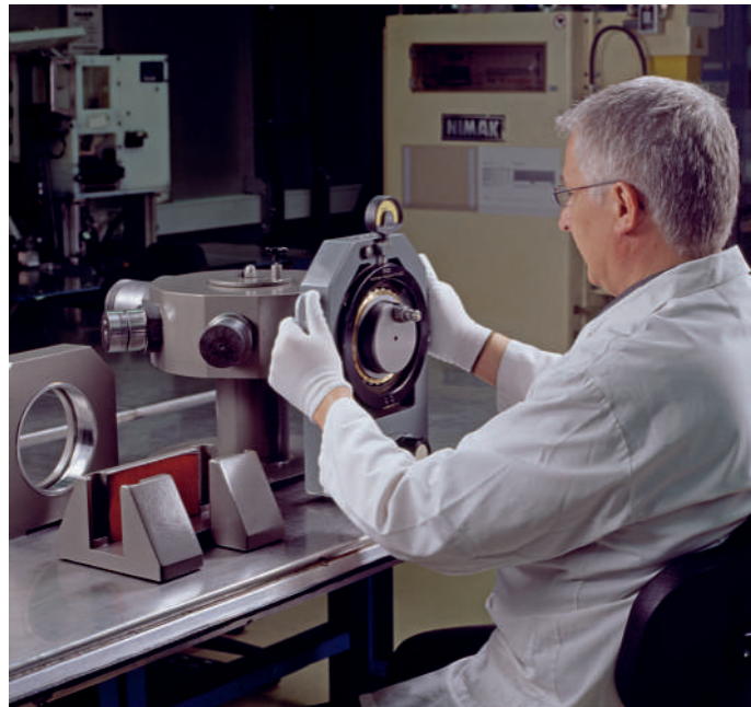
34 Positioning the enveloping circle gauge
