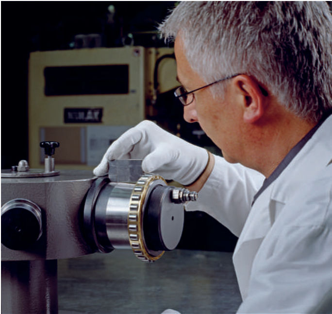
35 Measuring the spacing from the shaft shoulder
