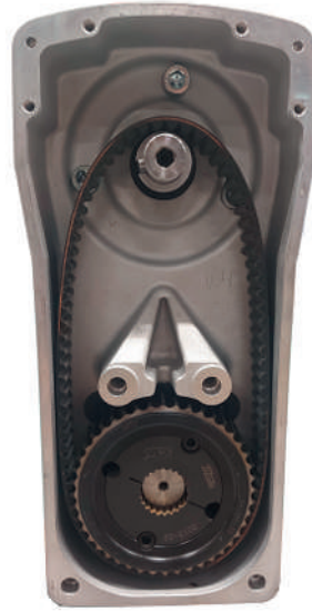
33 Belts around both pulleys with taper bushing
