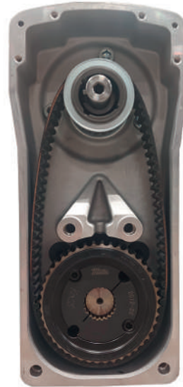
33 Belts around both pulleys with taper bushing
