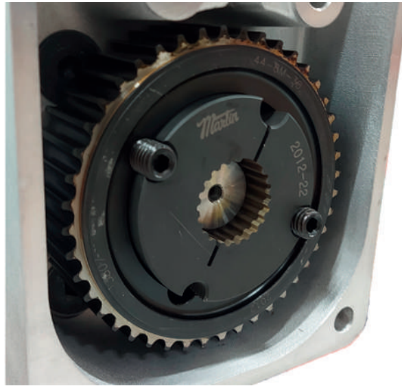
☞26 Pulley and taper bushing on the linear unit
