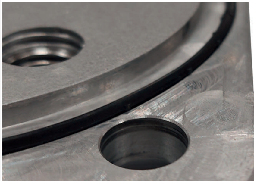
46 Alignment of the rubber seal
