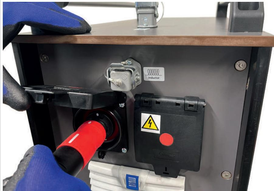
3. Applying axial pressure, press the plug deeper into the socket and turn the plug to the right, until it stops.
