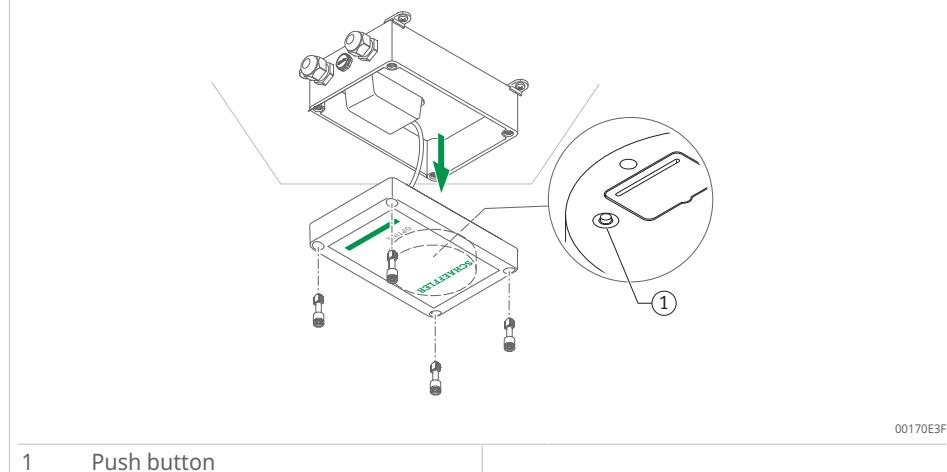
Pressing the push button starts configuration mode on the gateway ►54|7.
