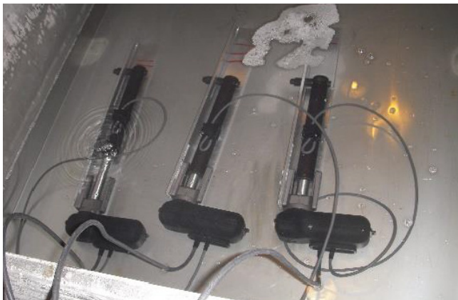
Complete actuator system exposed to ice water (ISO 16750-4) and Arizona dust (ISO 20653)
